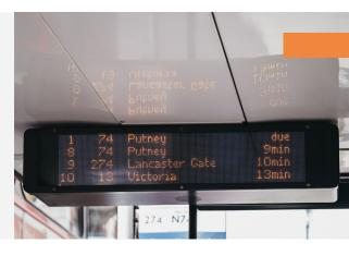
Filters used in conditions with a lot of direct light, such as sunlight or overhead light sources indoors, can benefit from anti-glare surface treatments to improve the readability of the display.
